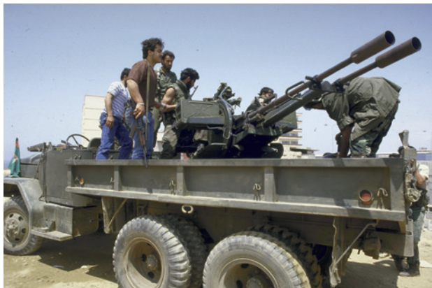
An Amal M35 'heavy technical' or 'gun-truck' mounting a 23mm ZU-23-2 AA cannon, West Beirut, 1985. All factions in Lebanon mounted the versatile ZU-23-2 on everything from light trucks to M113 armoured personnel carriers. (Photo by Bill Foley/The LIFE Images Collection/Getty Images)
