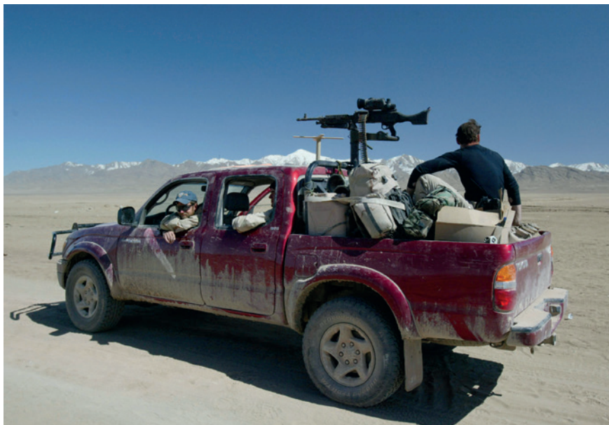
The iconic image of US Special Forces in Afghanistan driving a modified Toyota Tacoma near Gardez in early 2002. Note the aftermarket bull-bar, satellite communications (SATCOM) antennae on roof and 7.62mm M240B complete with what appears to be an AN/PAS-13 Thermal Weapon Sight. (Photo by Paula Bronstein/Getty Images)
