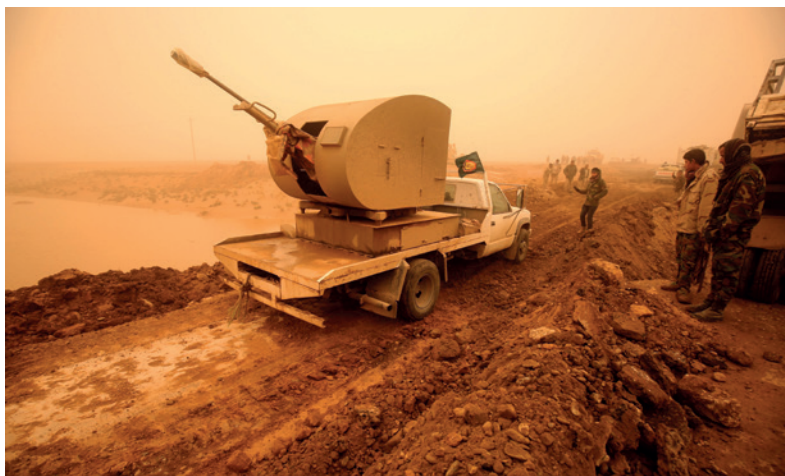
Pro-government Shia paramilitaries from the Popular Mobilisation Units (PMU) mounting a 23mm ZU-23-2 in a custom-made armoured turret, west of the Iraqi city of Mosul in 2016. The same turret has been mounted on heavily armoured commercial flat-bed trucks including tank-style vision slots and armour plating covering their tires. (Photo by Ahmad Al-Rubaye/AFP/Getty Images)
