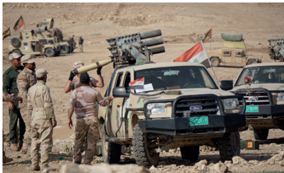
Iraqi soldiers loading an Iranian copy of the 12-tubed 107mm Type 63 MLRS mounted upon a Ford Ranger in Iraq 2017. The traditionally poor accuracy of such systems is improved by the use of quad-copter drones operated as aerial forward observers, a tactic used by both sides in the conflict. (Photo by Captain Timothy Irish, US Marine Corps)
