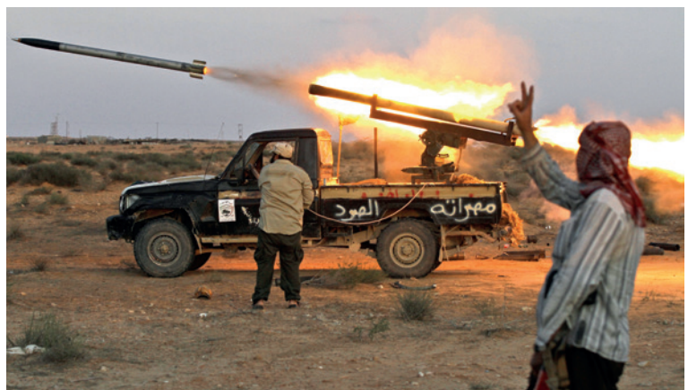
A spectacular shot of a just-launched 122mm Grad unguided rocket fired from an improvised mount upon a battered Land Cruiser, Libya, 2011. Although 57mm launchers are more common in the hands of Libyan militias, 107mm and 122mm rockets are also employed. (Photo by John Cantlie/Getty Images)
